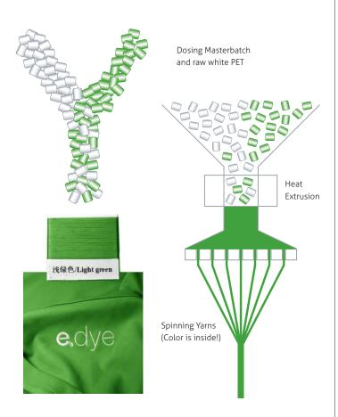
This process eliminates water consumption and reduces chemical use, energy comsumption and CO, emissions.
