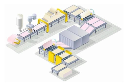
Raw materials are homogeneously mixed to form a gypsum slurry that is spread via hose outlets onto a paper liner on a moving belt conveyor. As second paper line is fed onto the production line from above to form the plasterboard. The plasterboard continues along the production line where it is finished, dried and cut to size.
