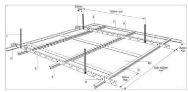
**SAS System 205** is a hook-on corridor suspended steel ceiling system; to facilitate access tiles are suspended at the perimeters using brackets and closure angles. A range of acoustic backing options provide up to 49dB acoustic attenuation or Class A acoustic absorption. For further details please visit <a href="https://www.sasintgroup.com/system205">www.sasintgroup.com/system205</a>
