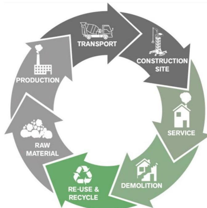
Figure 2: Stages of the life cycle of a product according to the analysis from "Cradle to gate" with options, module C1-C4, module D and optional modules.
