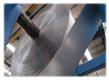
In the third process, the full-automatic double shafts slitting machine is fixed according to the desired ID (inner diameter), width, and length then finally the production of copolymer-coated aluminum tape is completed by slitting the master roll into tapes. Finally, the tapes are packed in accordance with the customer's specification and became ready for shipment. The aluminium used in the product comes mostly from Asia and Russia.
