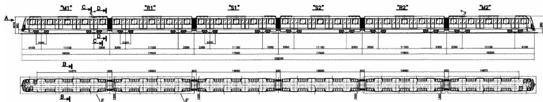
Metro Roma C consists of six carbodies with five articulations. The traction is supplied by sixteen electric engines, coupled on eight of the twelve bogies; the other four trucks are only trailers.
