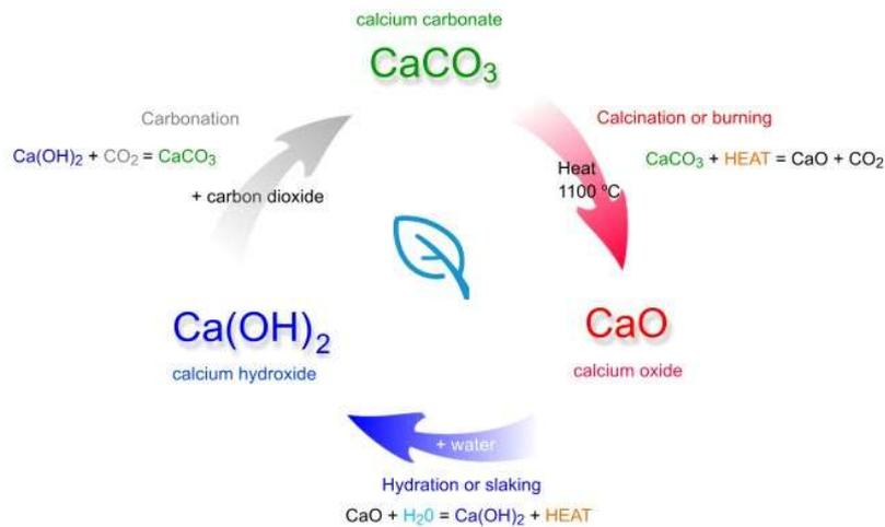
Figure 5. Lime cycle: Calcium carbonate-Calcium oxide-Calcium hydroxide.
