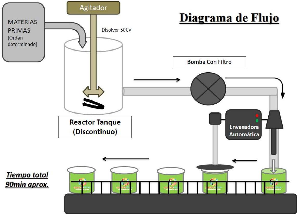
Figure 3. Graphene lime production process.
