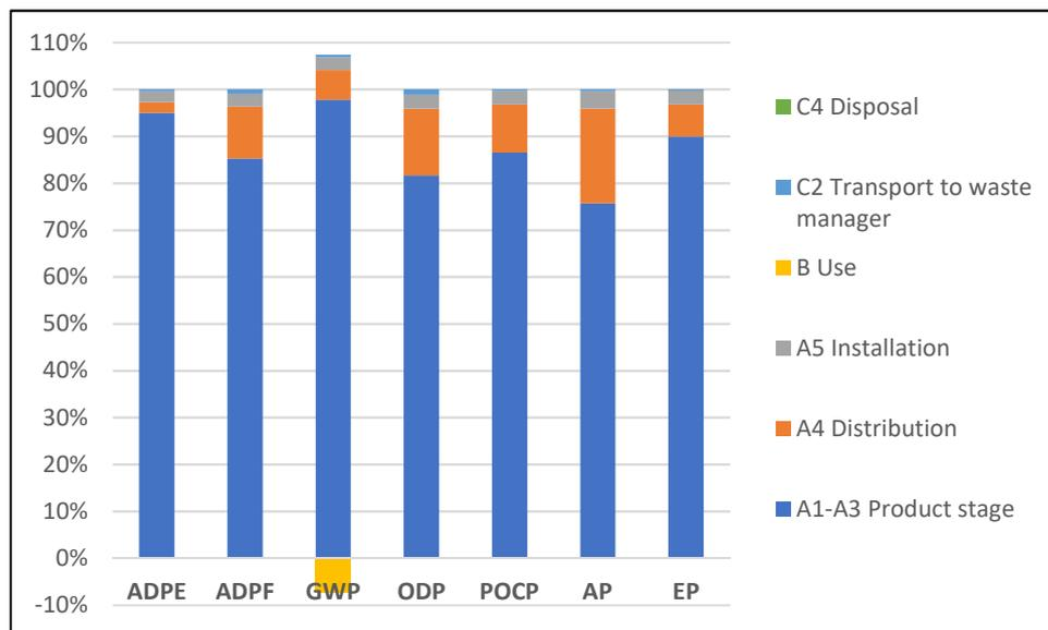
Figure 6. Potential environmental impacts of the life cycle of 1m<sup>2</sup> of Graphenstone® MortarFine Premium.
