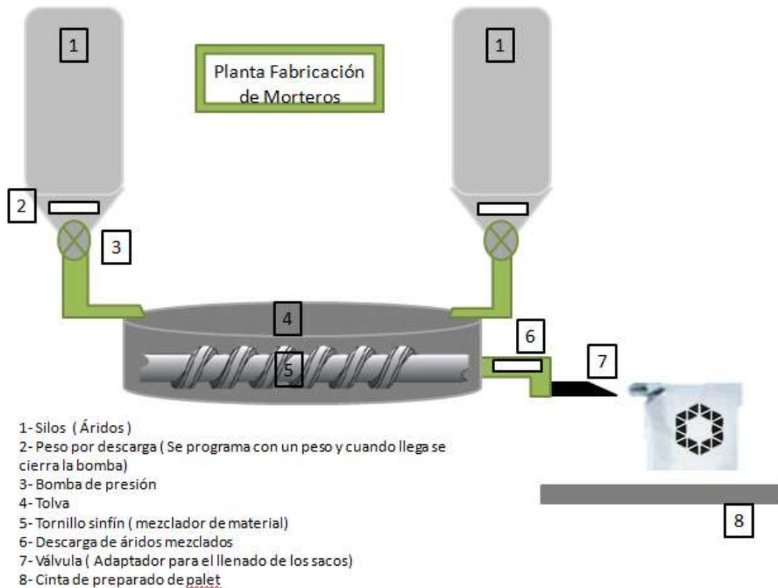
Figure 2. Aggregates production process.
