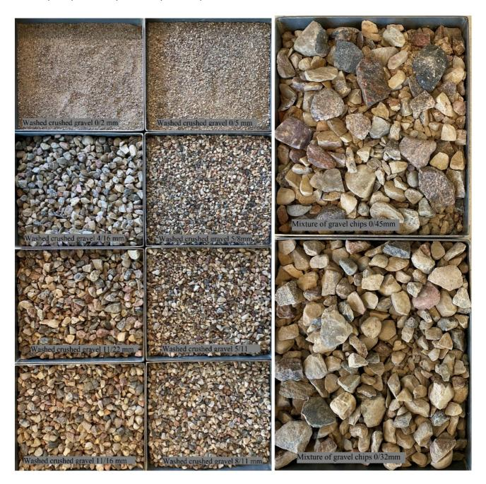
Aggregates are broadly used in industries for a different purpose. They are a primary component in the production of concrete and asphalt, but also serve as a filter and fill material or as a basic material for road building and railway construction.
