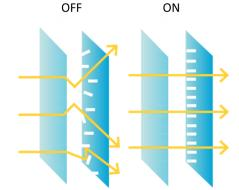
Figure 1 : simplified diagram of the operation of PRIVA-LITE
