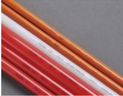
Rifeng PEX pipes are produced by crosslinked polyethylene which is obtained through a chemical process that increases the bonds between macromolecules to form a more complex structure than the normal polyethylene. Due to the crosslinking process, the strength of polyethylene is greatly enhanced and the excellent properties of crosslinked polyethylene have been proved to be a reliable
