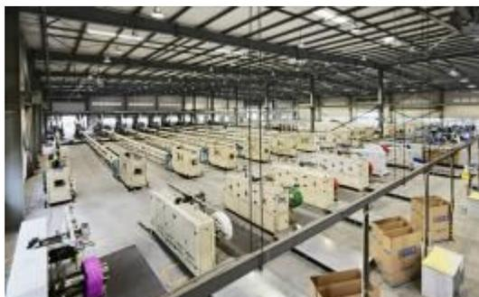
The screwed extruder as the main manufacture machine consists of extrusion, feeding, transmission, heating and cooling system as well as controlling system.
