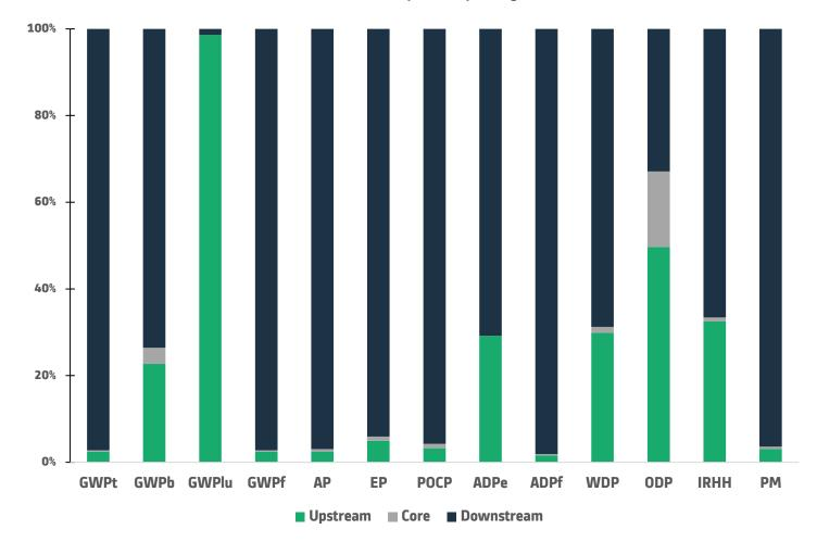
For most indicators, the downstream phase is responsible for the most significant part of the environmental impacts. This is especially due to the electricity consumption for traction and auxiliaries during the use of the metro for the 35 years of its expected lifetime.
