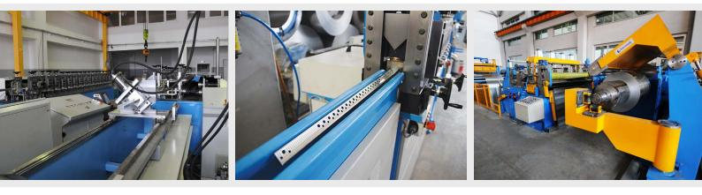
The products are manufactured from hot dip galvanized carbon steel. Purchased galvanized coils are divide into narrower bands whose width fits the specific profiles and accessories. Then, steel profiles are manufactured through roll forming technique while accessories are cut from bands according to relevant specifications.
