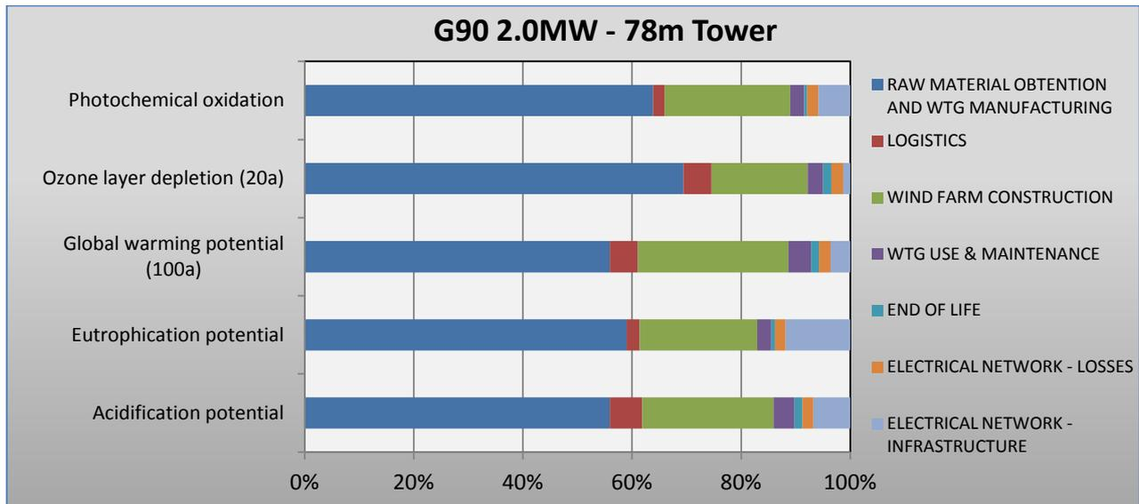
As shown in the figure above, the environmental impacts are mainly caused in two of the stages within the energy life cycle, which are the WTG manufacturing and the construction of the wind farm infrastructures.
