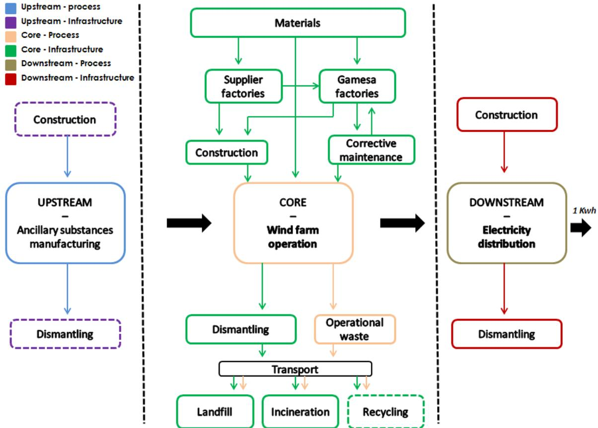
The blocks in the graph above whose boundary is a dashed line, have not been taken into account in the LCA, as permitted by the associated PCR. The arrows represent the different transport stages for the materials, parts or bigger components.
