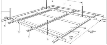
SAS System 200 is a hook-on suspended steel ceiling system; a range of square, rectangular, trapezoidal and triangular are supported from a concealed J-bar suspension rail. A range of acoustic backing options provide up to 49dB acoustic attenuation or Class A acoustic absorption. For further details please visit www.sasintgroup.com/system200
