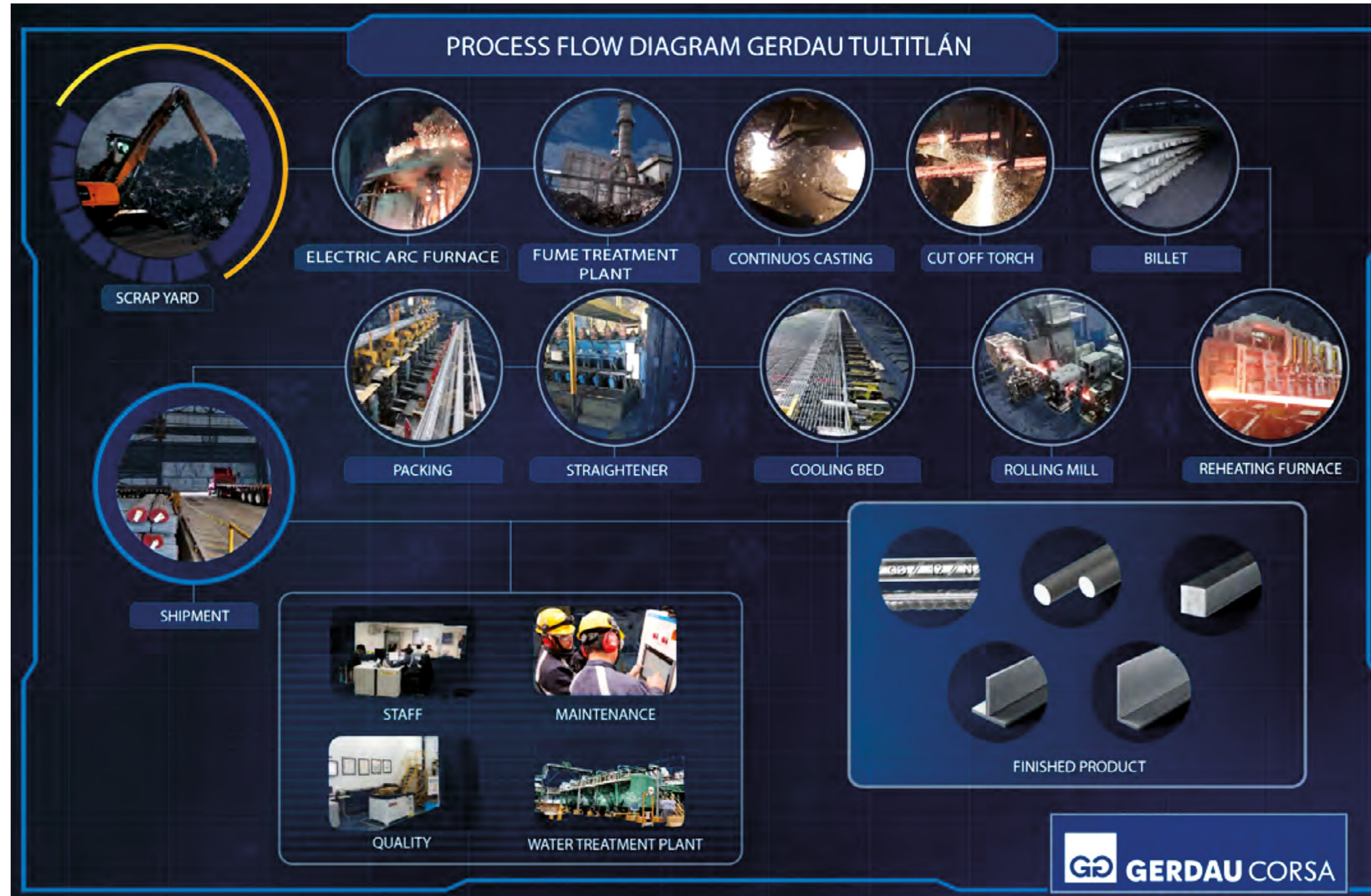
Figure 1. Flow diagram of steel slag (co-product)
