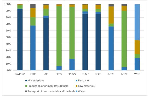
The LCA of CEM I cement in the UK is mainly influenced by the following factors, which vary from cement plant to cement plant:
