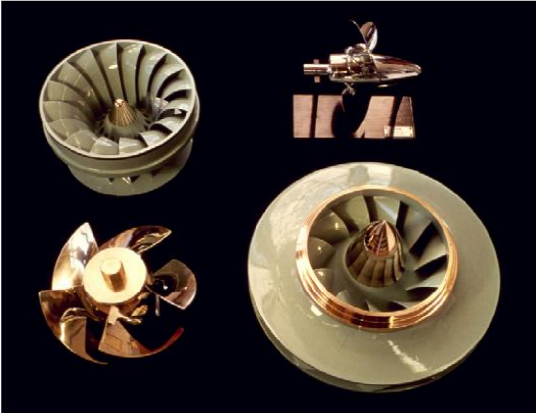
Figure 6 Runners for Kaplan turbine (upper left), Propeller turbine (upper right), Francis turbine (lower left), Francis turbine for high heads (lower right).
