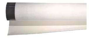
Synthetic membrane made of flexible modified polyolefins, obtained by co-extrusion, UV resistant, reinforced with fiber glass mat, laminated on the lower face to a nonwoven felt.
