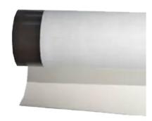
Synthetic membrane made of modified polyolefin TPO obtained by co-extrusion, UV resistant with polyester mesh insertion and laminated on the lower face to a nonwoven felt.
