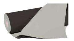
Synthetic membrane, made of flexible modified polyolefin TPO, obtained by co-extrusion, UV resistant, stabilized by fiber glass mat.
