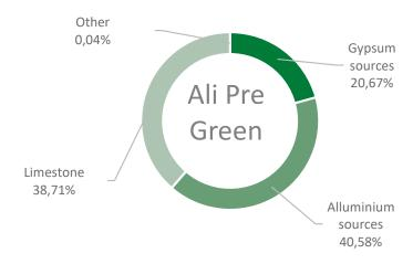
**ALI PRE GREEN** contain a high percentage of recycled materials used as aluminum sources. This particularity implies savings in natural resources and energy which would otherwise have been consumed. The aluminum based recycled materials result from the production of secondary aluminum and as such are classified as pre-consumer recycled materials according to the standard ISO 14021. Following rules set in this standard, the recycled material content of **ALI PRE GREEN** at 46.8%.
