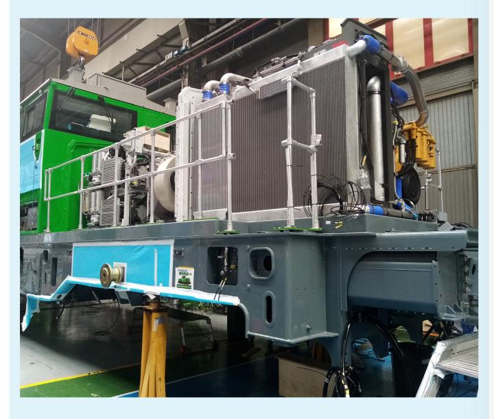
Furthermore, the DR19 diesel engine exhaust emissions comply with the EU Stage V "Regulation (EU) 2016/1628 on requirements relating to gaseous and pollutant emissions limits and type-approval for internal combustion engines for non-road mobile machinery, including railway vehicles".
