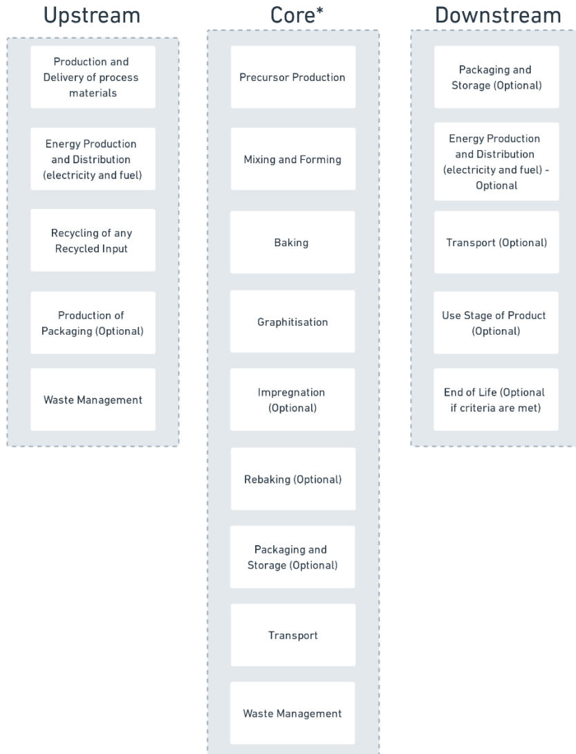
Figure 4 details the system boundary for an EPD on synthetic graphite produced for electrodes.
