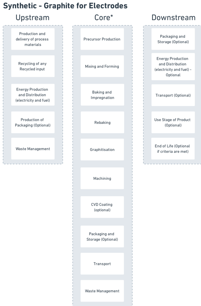
Figure 3 details the system boundary for an EPD on synthetic graphite produced for electrodes.
