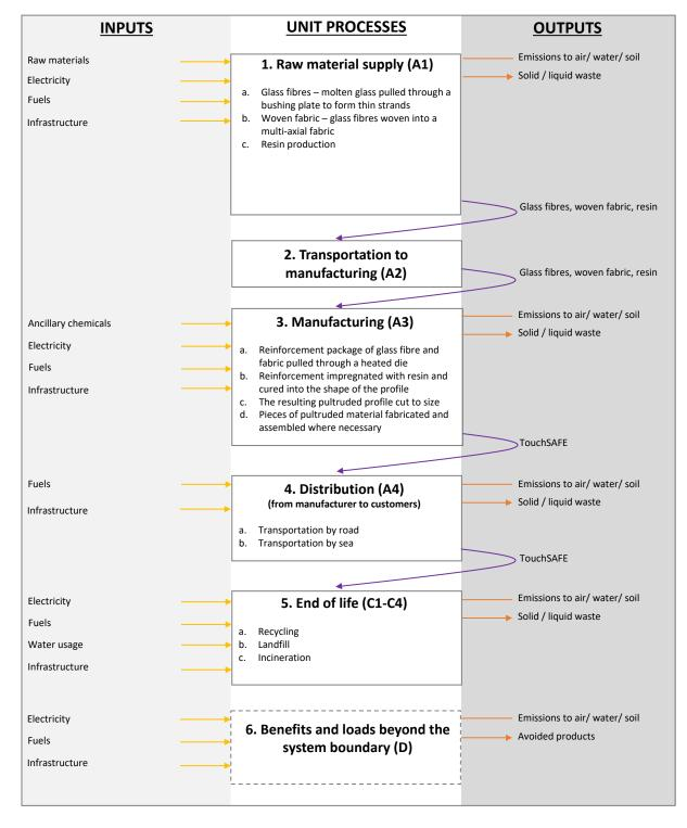
Yellow line = input of material/energy, orange line = output of waste/direct emission, purple line = output of product/co-product, arrowhead on line = transportation stage considered.
