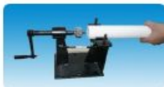
Step 1: Pipe cutting
