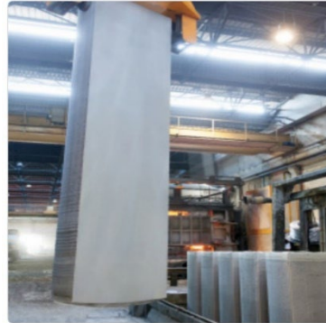
Figure 3. 5 meters long aluminium post-consumer recycled slab.
