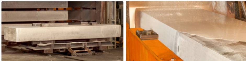
Figure 4. The slabs are scalped to clean the surfaces and introduced in to a gas oven for preheating and homogenizing the milled slabs prior to been prepared for the hot rolling process.
