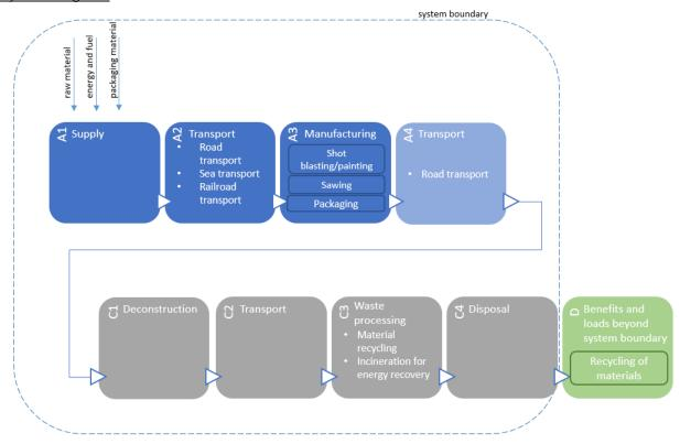
The pretreatment and processing of Carbon steel long products includes blasting/protective finishing and sawing. 32% of the Carbon steel long products are being processed and of that, 70% is sawing and 30% blasting/protective finishing.
