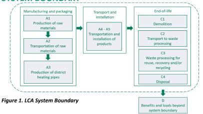
This EPD is "Cradle to gate with options, modules C1–C4, module D and with optional modules"
