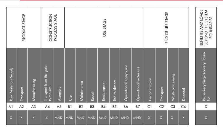
The system boundary covers the production of raw materials, all relevant transport down to factory gate, manufacturing by AGT, deconstruction of the product from its construction site, transport of the deconstructed material to waste processing facility with an assumed distance of 200 km, waste processing and disposal.
