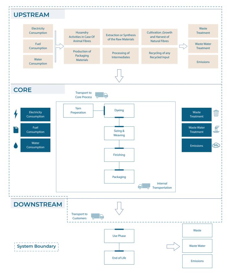
The International EPD® System has adopted an LCA calculations procedure, which is separated into three different life cycle stages:
