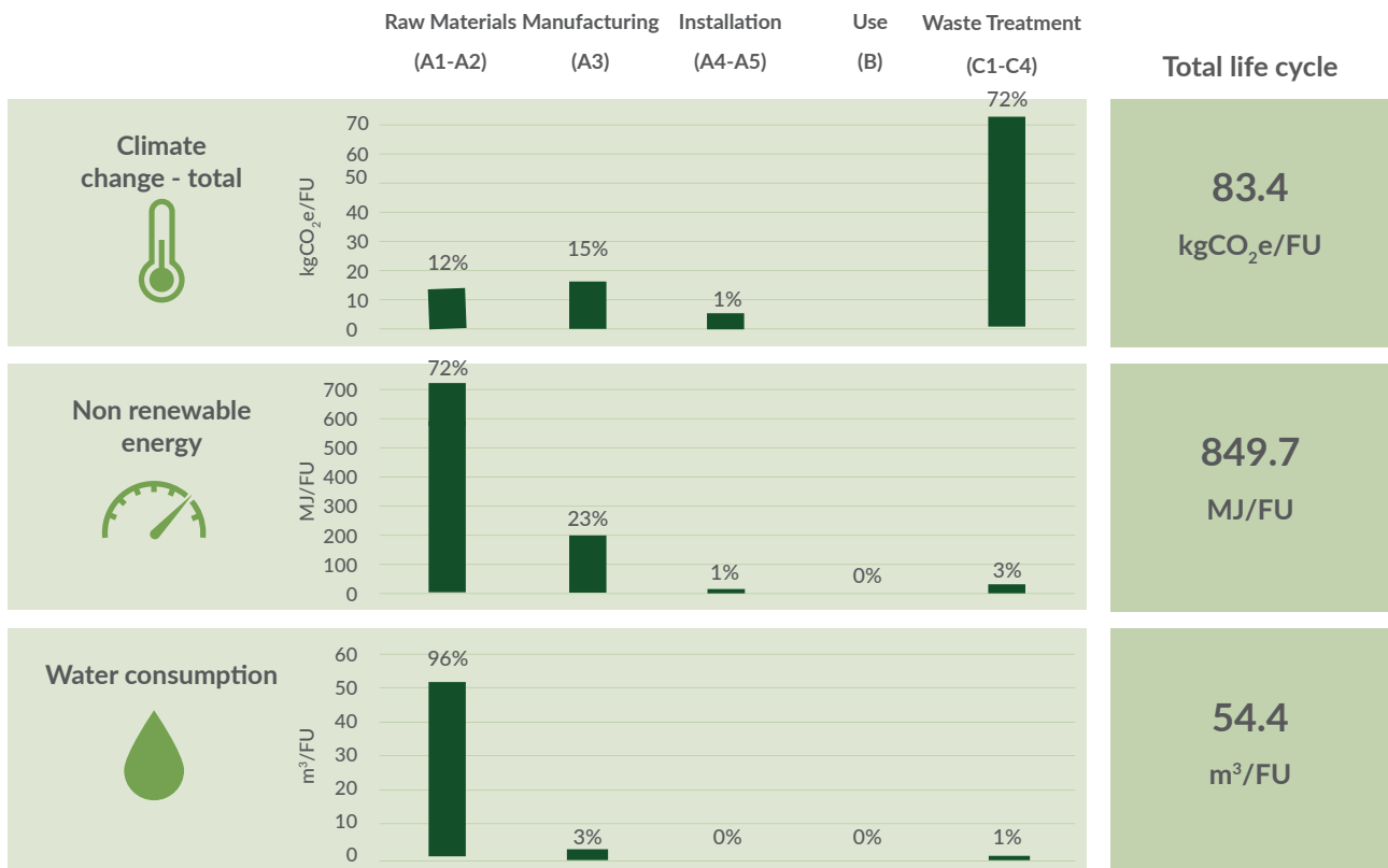
Figure 1: Summary of the impact of life cycle stages on three key environmental impact categories
