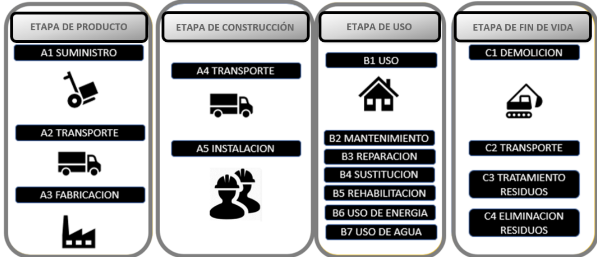
Figure 2: Stages of a product's life cycle according to cradle-to-grave analysis.
