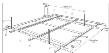
**SAS System 130** is a modular lay-in steel ceiling system; tiles are supported from SAS Alugrid or SAS Tee Grid. Alugrid-Q features a continuous linear recess with an M6 thread while providing a completely flush ceiling. Alugrid-P is a plain version without the threaded recess; Tee Grid provides a tegular effect. A range of acoustic backing options provide up to 45dB acoustic attenuation or Class A acoustic absorption.
