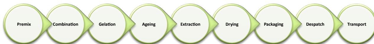
Spaceloft® Production Process
