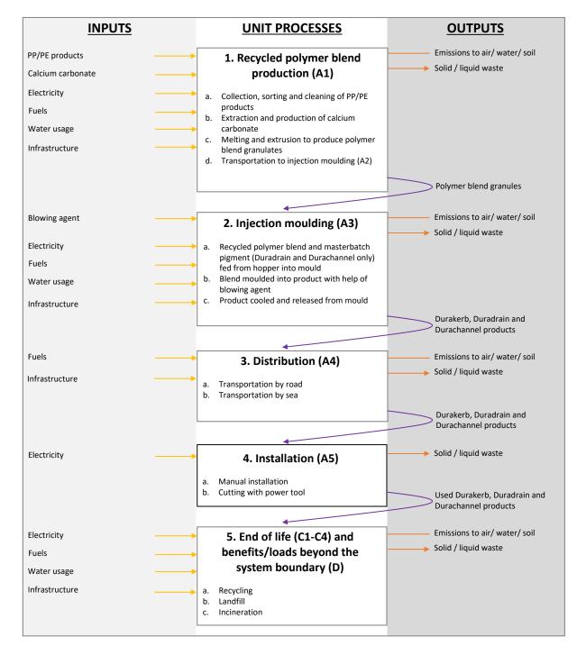
Yellow line = input of material/energy, orange line = output of waste/direct emission, purple line = output of product/co-product, arrowhead on line = transportation stage considered.
