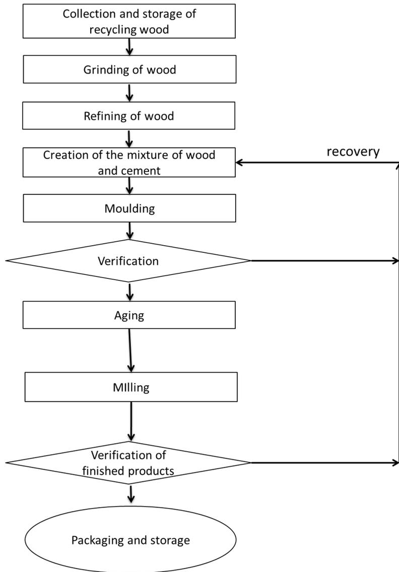
Figure 2: Production process of the ISOTEX® wood cement acoustic elements
