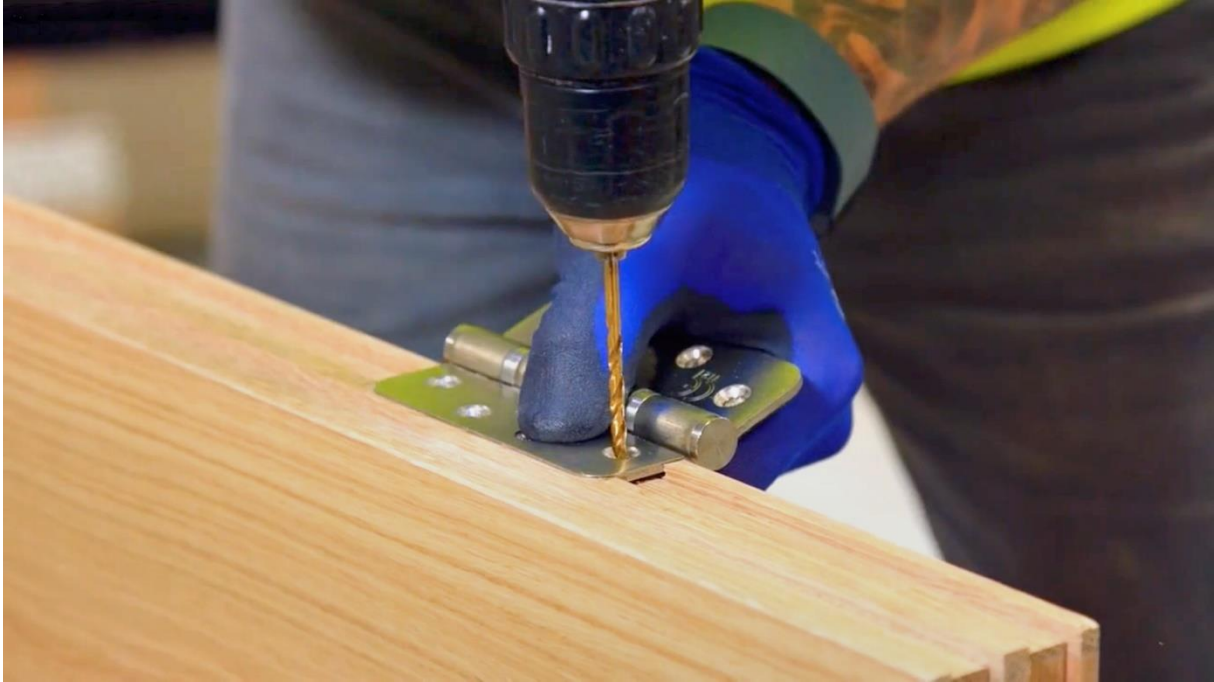
Figure 4: Generic example of fitting the hinges
