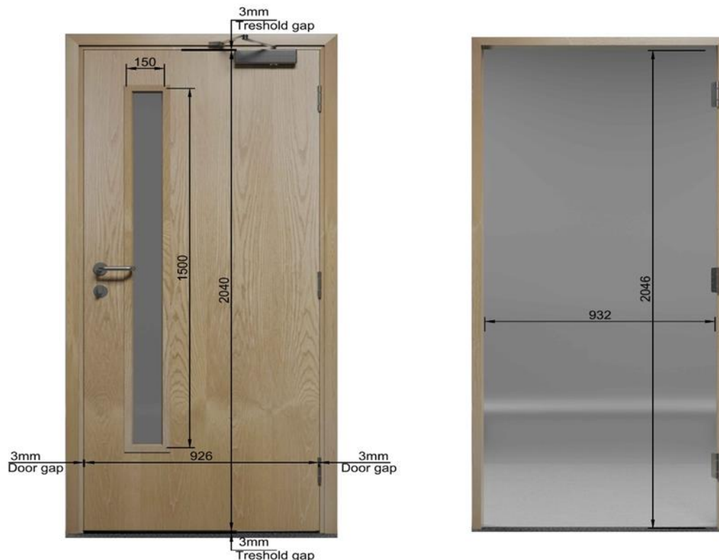
Figure 1: Dimensions of door and required door frame
