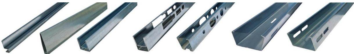
Profiles requiring long-term corrosion resistance are manufactured from sheets with a special ZnAlMg surface treatment. The product provides up to four times the corrosion protection, although less zinc is used in its production compared to conventional products.
