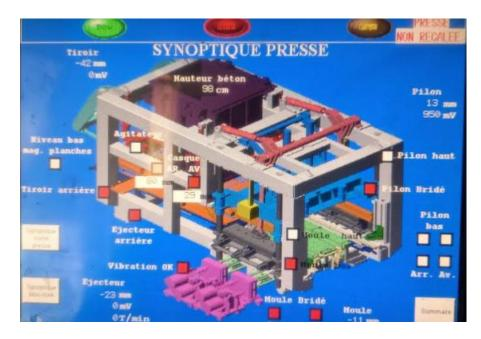
Concrete blocks are produced using a vibrating press. These are automatic machines with a high production rate that are integrated in a production unit that includes the mixing, the press, the curing area and the conditioning. The production includes the 4 process as follows:
