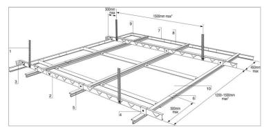
**SAS System 120 - Aluminium** is a modular clip-in aluminium suspended ceiling system; Square and rectangular clip-in metal ceiling tiles are supported from a concealed SAS suspension grid. A range of acoustic backing options provide up to 42dB acoustic attenuation or Class A acoustic absorption. For further details, including the dimensions of the individual grid items, please visit <a href="https://www.sasintgroup.com/system120">www.sasintgroup.com/system120</a>
