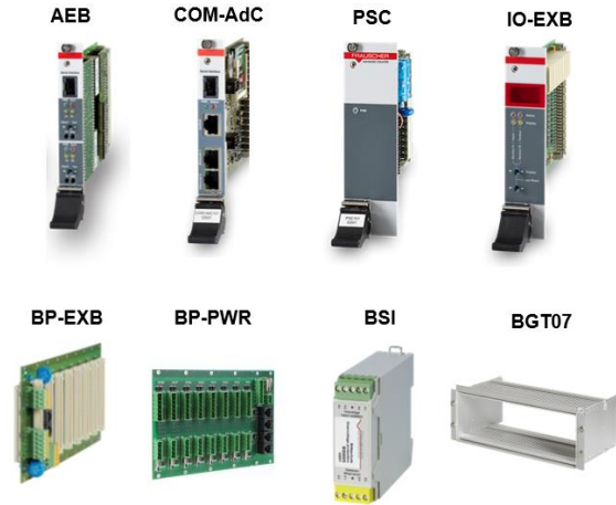
Figure 1: Overview of the 7 modules and the casing forming a complete Indoor installation.
