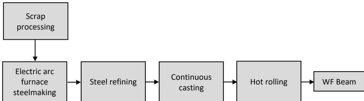
Figure 1. Flow diagram of steel WF beam manufacturing process
