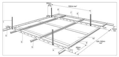
**SAS System 120** is a modular clip-in steel suspended ceiling system; Square and rectangular clip-in metal ceiling tiles are supported from a concealed SAS suspension grid. A range of acoustic backing options provide up to 42dB acoustic attenuation or Class A acoustic absorption. For further details, including the dimensions of the individual grid items, please visit <a href="https://www.sasintgroup.com/system120">www.sasintgroup.com/system120</a>
