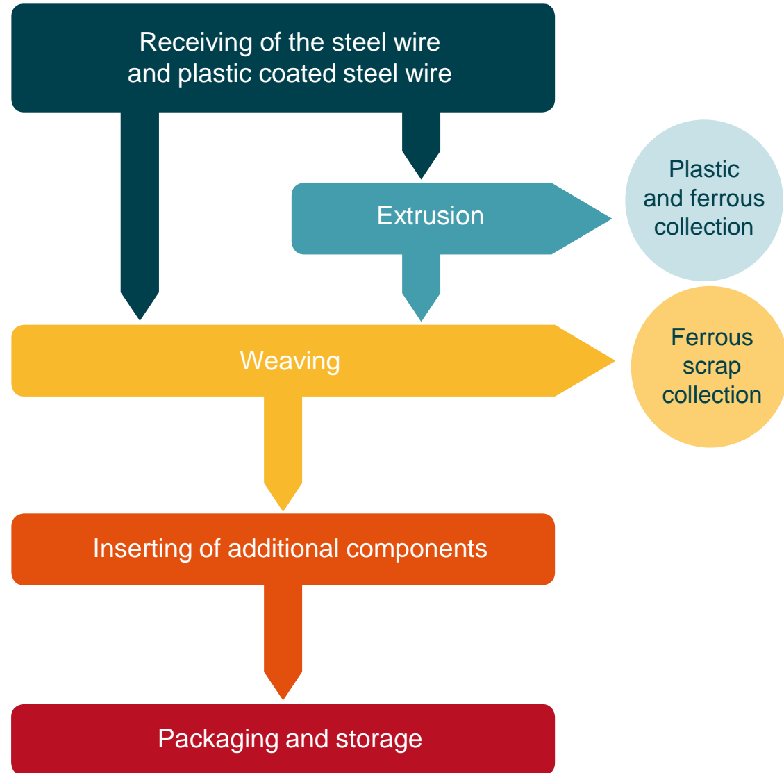
Figure 4: Production process of the Gabions
