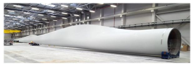
Figure 4: Blade manufacturing in Siemens Gamesa
