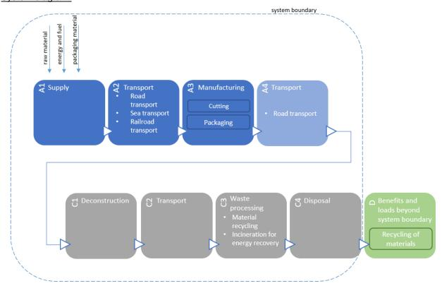
The steel coils coming from the suppliers are cut to the desired length into sheets or alternatively slitted lengthwise into a narrower coil. The top layer is usually scrapped from the start of the coil if it has dents/scratches. Also, a certain part of the end of the coil is usually scrapped. The cut sheets and slitted coils are packed on wooden pallets. Packages are protected with cardboard corner protectors. The packages are tightened with a plastic/steel band.
