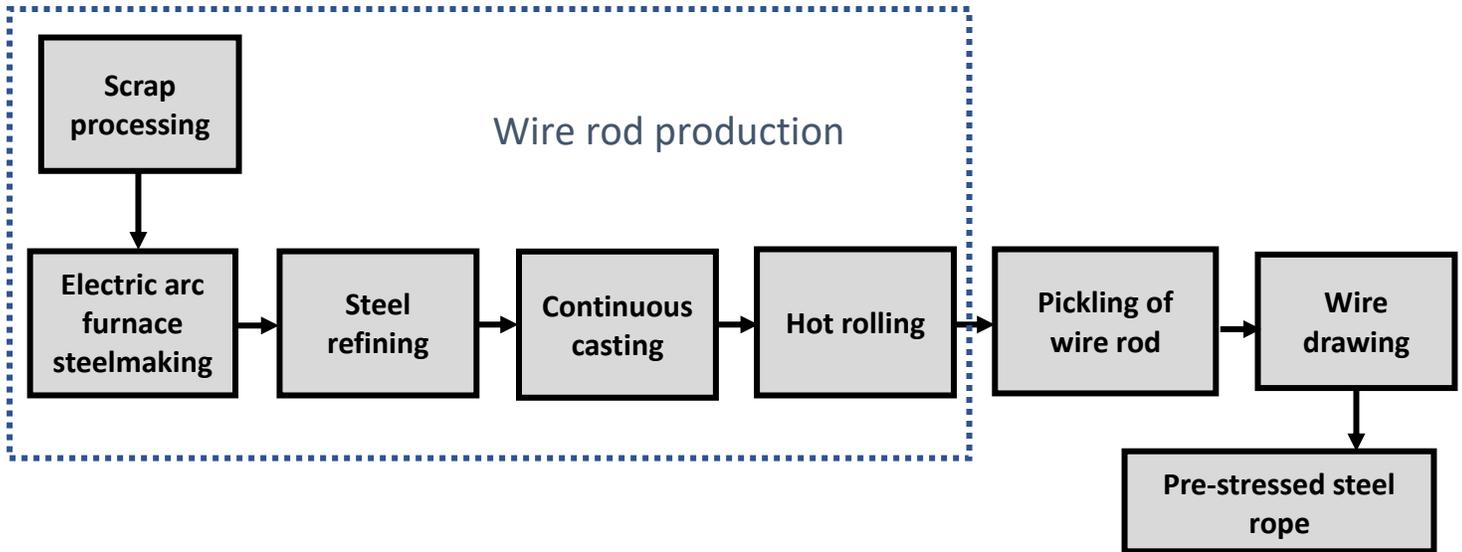
Figure 1. Flow diagram of the manufacturing process of pre-stressed steel rope.
