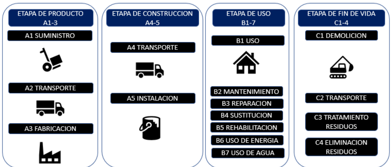
Figure 2: Stages of the life cycle of a product according to the "cradle to the grave" analysis.
