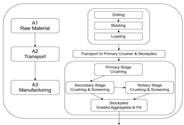
Delivery to Client via Truck or to Asphalt, Concrete Blocks & Ready Mix Plants via Conveyors
