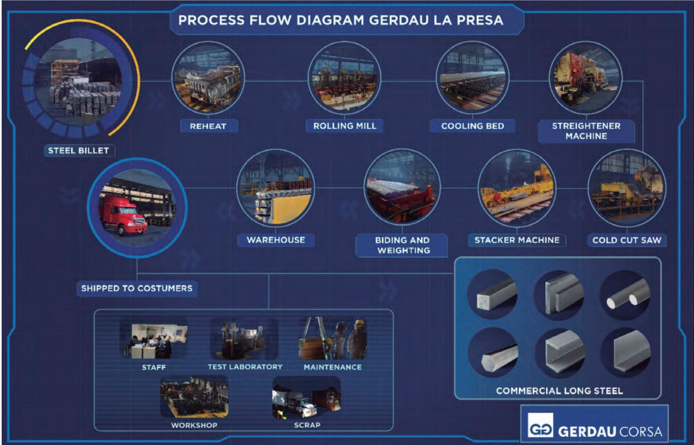
Figure. 1. Commercial long steel hot-rolled manufactured from steel scrap.
