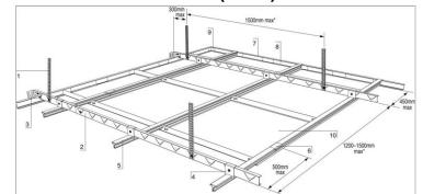
**SAS System 205-Aluminium** is a hook-on corridor suspended aluminium ceiling system; to facilitate access tiles are suspended at the perimeters using brackets and closure angles. A range of acoustic backing options provide up to 49dB acoustic attenuation or Class A acoustic absorption. For further details please visit <a href="https://www.sasintgroup.com/system205">www.sasintgroup.com/system205</a>
