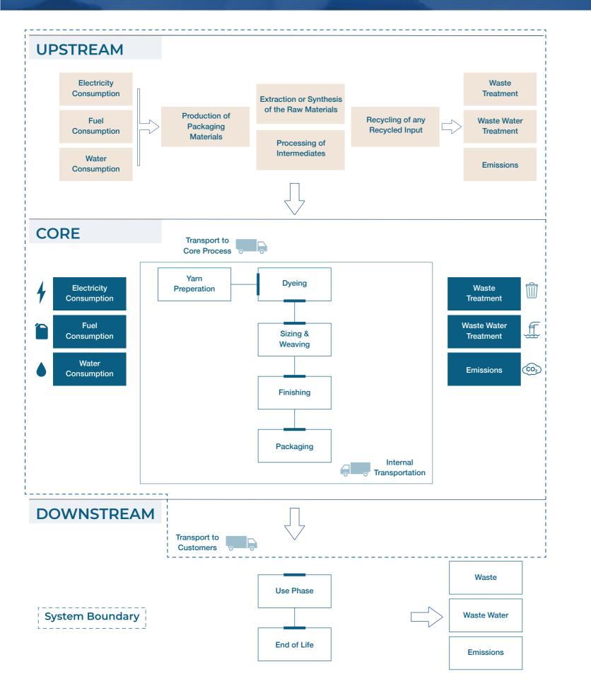
The International EPD<sup>®</sup> System has adopted an LCA calculations procedure, which is separated into three different life cycle stages:
